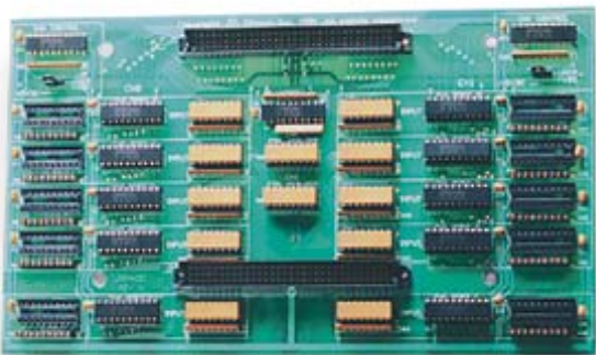
The HVCX1 option is user-configurable as either input or output in 8-channel multiples
